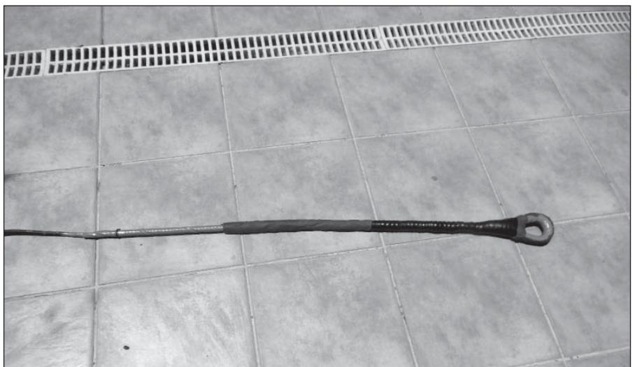
Figure 8 — A Phillystran big grip and stainless thimble after blue epoxy coating and showing progressive potting and taping, left to right.
