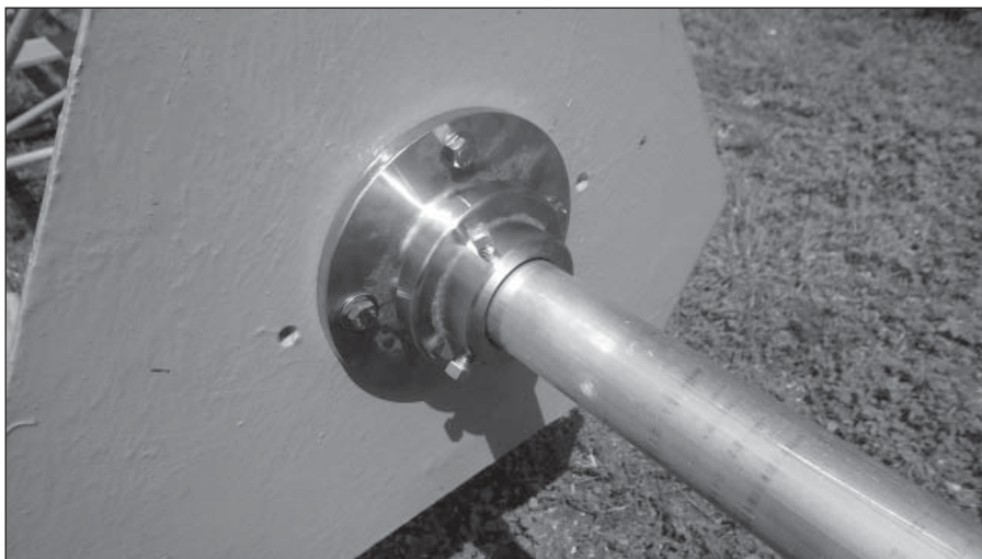
Figure 5 — A stainless-steel thrust bearing and aluminum mast at a tower top plate.
