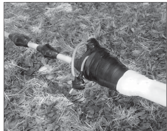
Figure 14 — The mast-base junction and matching assembly of a Ringo Ranger 2-meter vertical, properly potted and taped.
